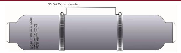
Carrying Handles and End caps enable the user to safely transport pressurized samples.
