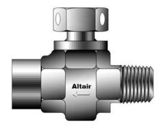
Rupture disc is an inexpensive safety device that protects the sampling cylinder from over pressurization by venting the cylinder contents in atmosphere. Rupture disc assemblies are machined from SS 316 ASTM A479 bar stock. Rupture disc are made of SS 316, with PTFE/Viton® seals. Relief valves are provided instead of rupture disc where application requires re-closure after venting of over pressurized fluid.
